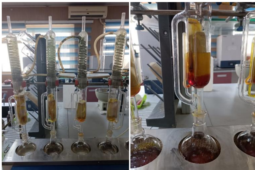
Figure 1: Soxhlet apparatus used for turmeric extraction.
